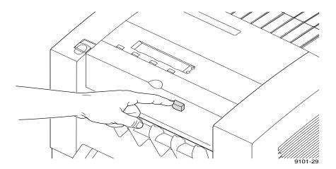
4. Using both hands, pull the jammed media out the top of the printer.
