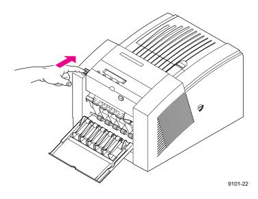
3. If necessary, open the exit cover using the blue release button located inside the front cover, at the top of the printer.
